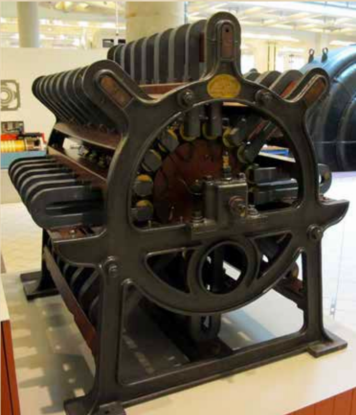
ABOVE: A magneto generator of 2kW made by the Société de l'Alliance around 1870.
